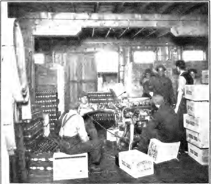
FIG. 34.—SALMON CAN-LABELING MACHINE
